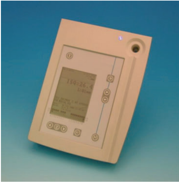
Fig. 10. The third generation and the first commercially available resonance frequency analysis equipment (Ostell™).
