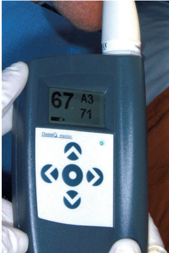
Fig. 14. In several implant systems, the Mentor™ gives one low and one high implant stability quotient value, reflecting the highest and the lowest level of stability of an implant.
